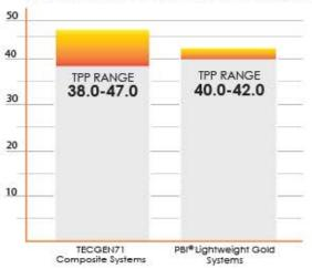
TECGEN71 fabric enables the use of significantly lighter composites without sacrificing thermal protection.
